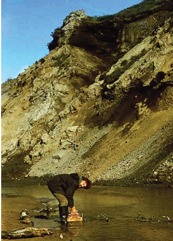
Figure 4 We screen sediments in the field, using a large handmade box with 0.5 mm mesh sieve, letting river, lake, or pond water in and out through the sieve only. The screening is aimed at removing most, but not all of the mineral component, so some amount of silt remains in the box, helping preserve the shape of many fossils smaller than 0.5 mm that might otherwise be lost. These specimens usually float on top of the silt and remain in the sample.
